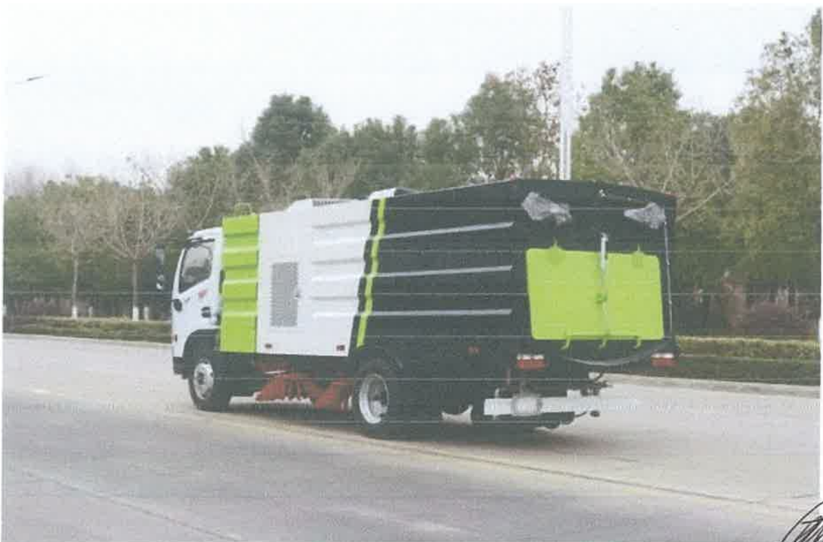
cleaning device: middle four-disc sweep + rear suction nozzle
